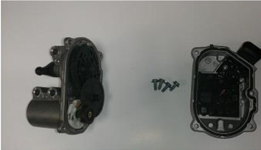
Step 3. Further disassembly is needed. You have to take the motor out by removing the little plastic cap that holds the rotor in place. Later you can remove the rotor which then lets you remove the motor itself by unscrewing two bolts.
