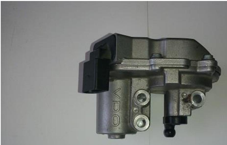
Step 2. You will need to take the apart in order to complete the installation. 4 bolts have to be unscrewed, unscrew them using a Torx T20.
