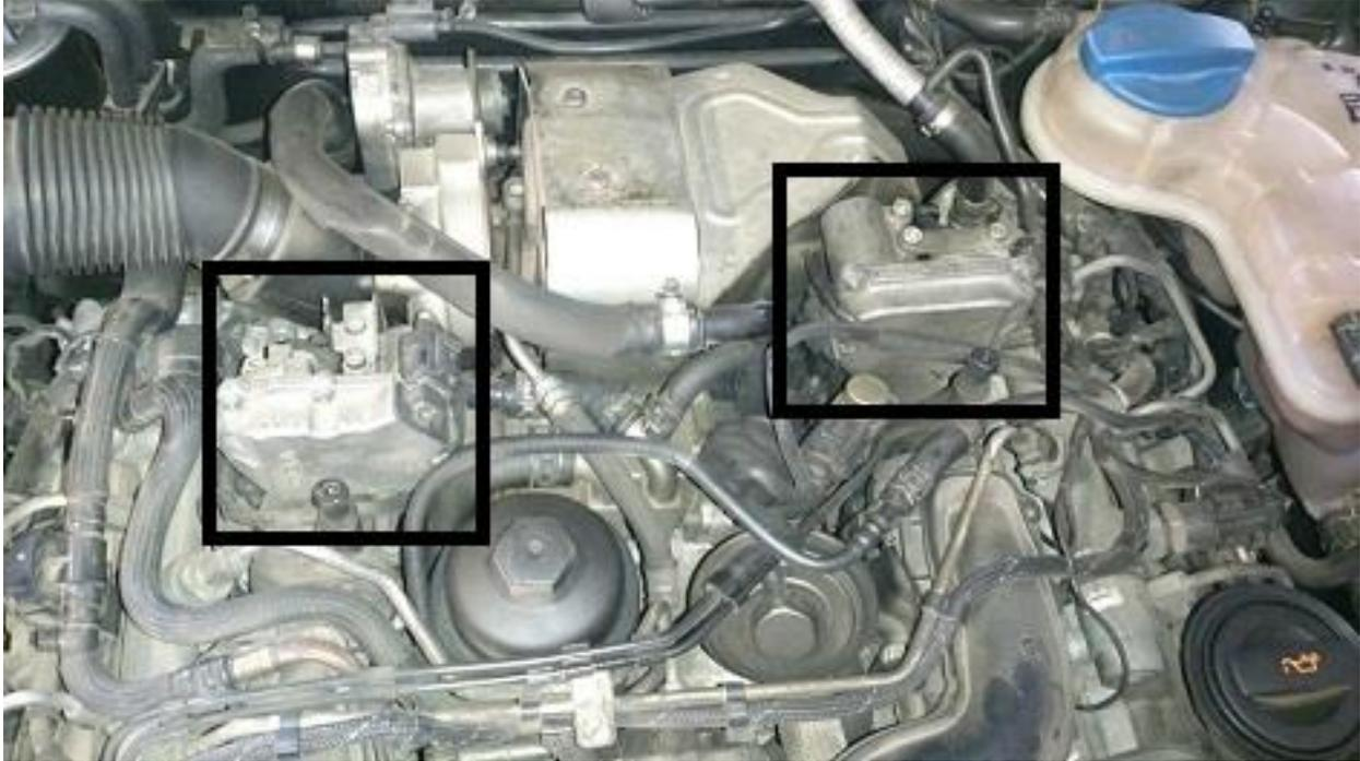
The inlet manifold flap motors are clearly marked. Undo the bolts and remove the flap connector. Remove them from the engine bay.
